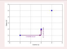
Graphical representation of  $\gamma^1 \delta^1 \oplus \gamma^3 \delta^2 \oplus \gamma^4 \delta^5 \in \mathbb{B} [\
